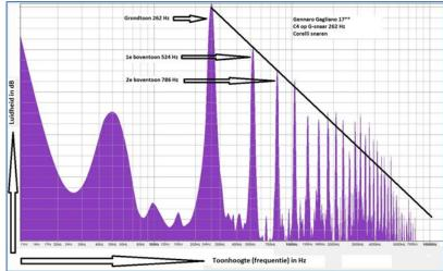
remains below the black line, the overtone is weaker. If the peak is above the line, then that peak is proportionally stronger (louder). The part to the left of the root is not important for the violin, and should therefore not be interpreted in that context. These are the sounds of the computer, including the 50Hz tone caused by the frequency of the mains.
