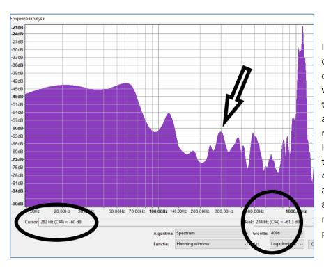
In the oval at the bottom left of the image we read that the cursor, shown as a white vertical line just to the left of the black arrow, is at 282 Hz and in the circle at the bottom right that the peak is at 284 Hz. In the same circle we read that the resolution (Size) is at 4096. It is clearly visible in the audiogram near the black arrow that the peak is not really peaked, as with the next peak to the left.
